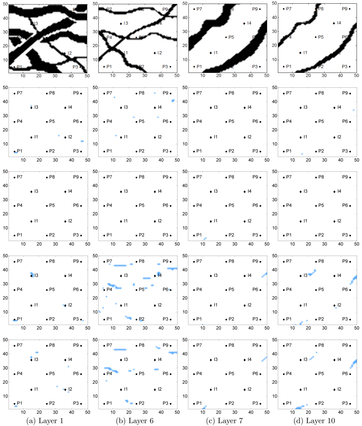
Figure 4.39: 0% probability maps of sand channels (Case 2.2, N_e = 500 ): true (1st row); posterior, TD, 20 \times 20 \times 5 \times 1000 (2nd row); posterior, TD, 37 \times 36 \times 8 \times 778 (3rd row); posterior, NTD, 20 \times 20 \times 5 \times 1000 (4th row); posterior, NTD, 37 \times 36 \times 8 \times 778 (5th row).
