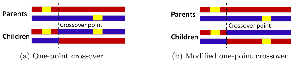
Figure 3.4: Illustration of the original one-point crossover and the modified one-point crossover. The red and blue colors represent \mathbf{x} of the two parent chromosomes respectively. The yellow color corresponds to a specific gene unit \mathbf{x}_j^b, j = 1, 2, \dots, N_w .
