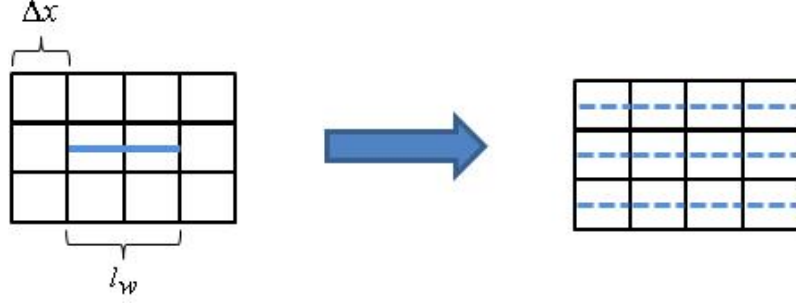
Figure 5.6: Schematic of a horizontal well by distributed perforations.
